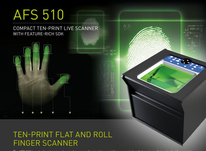
The AFS 510 is a sturdy yet compact, easy-to-use, professional ten-print live scan solution that captures flat and rolled fingerprints. It provides fast, forensic-quality fingerprint capturing, enrolled fingerprint images comply with U.S. strict biometric standards: the FBI IAFIS IQS Appendix F.
